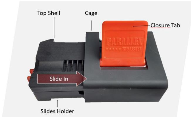
3. Push down the closure tab to compress the pogo pin and bring the slides together. Wait 10 sec.
